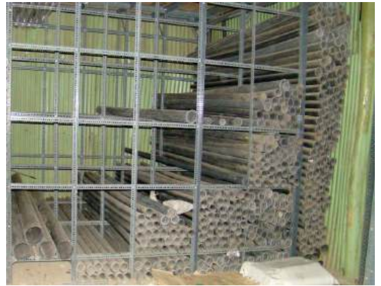
Slotted Angle Pipe Racks
