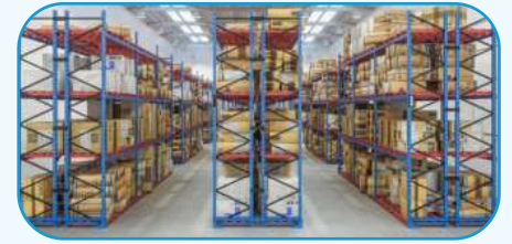
Narrow Aisle Pallet Racking
